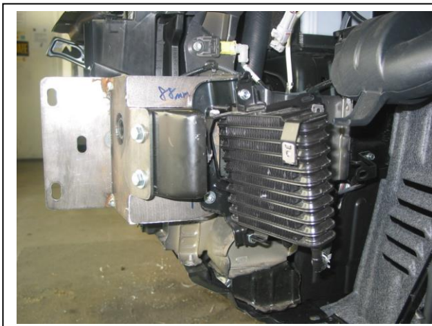
Figure 5: Oil cooler mounted to passengers side outer.
