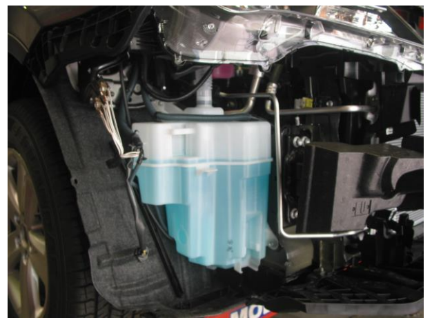
Figure 2: Disconnect bottle from passengers side inner guard
