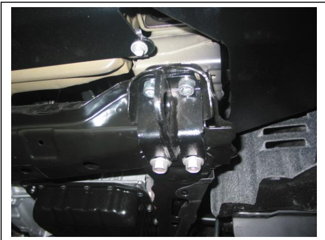
Figure 15: Tow hook installed onto under body frame
