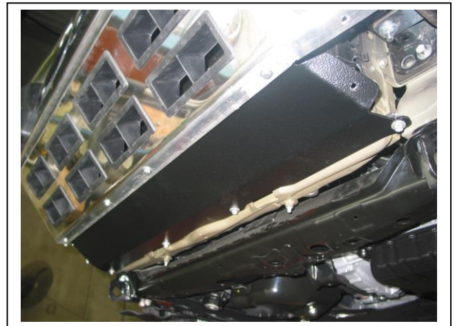
Figure 16: Centre under body guard fitted
